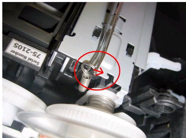
8) Connect the springs on each side of the spur holder to the switch system unit and the purge drive system unit respectively.
